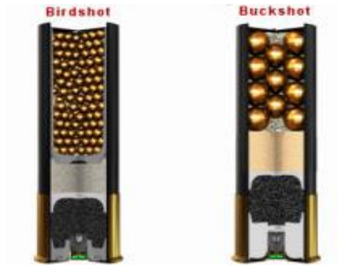
Figure 29. Cross section of two shotgun shells and their main components loaded with small pellets (“birdshot”) and, respectively, large pellets (“buckshot”) (taken with permission from Beiglböck and Walzer 2019).
