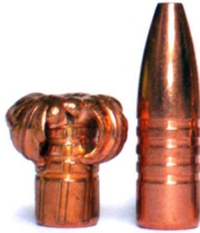
Figure 27. The shape of a deforming bullet before (right) and after hitting a body (left). Note the typical “mushroom shape” ensuring high energy-transfer in the body (Beiglböck and Walzer 2019).
